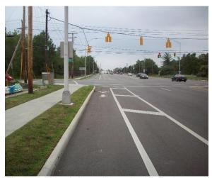
Figure 3. A bicycle lane with a striped buffer in Hilliard, Ohio.
